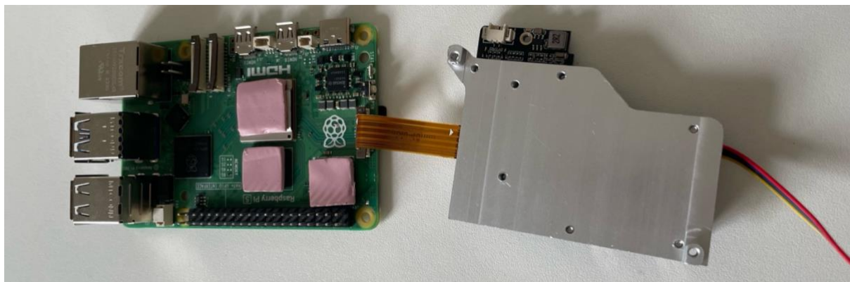
Figure 13. Insert the PCIe ribbon from the Waveshare board into the PCIe connector on the Raspberry Pi and close the PCIe gate to hold it into position.
