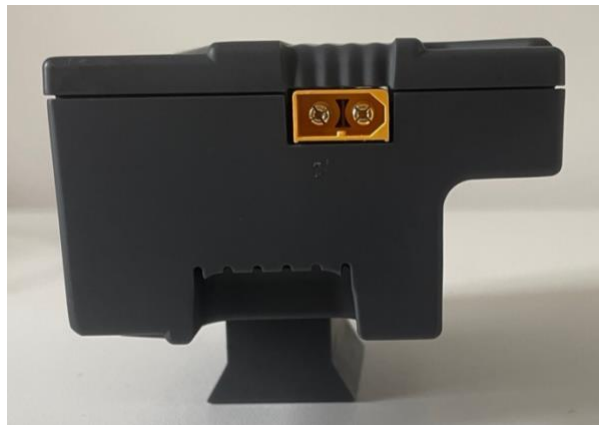
Figure 22. AStarBox with finder foot attached to the aluminium puck on the base of the box.
