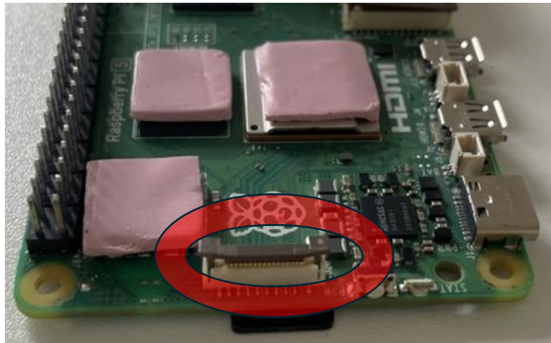
Figure 12. Lift the gate on the PCIe connector – this allows you to connect the Waveshare board.
