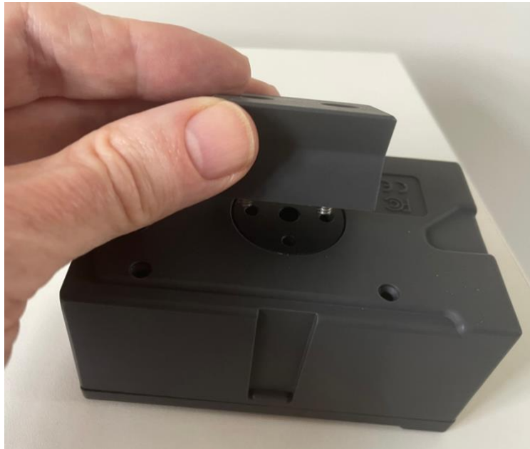
Figure 21. Installing the finder foot attachment. Place the two M4 screws into the bottom of the finder foot and align with the holes in the aluminium puck.
